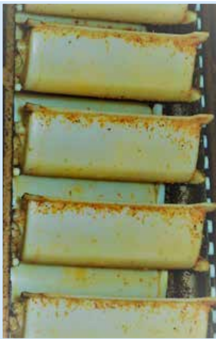
Open chain contaminated by food soil
