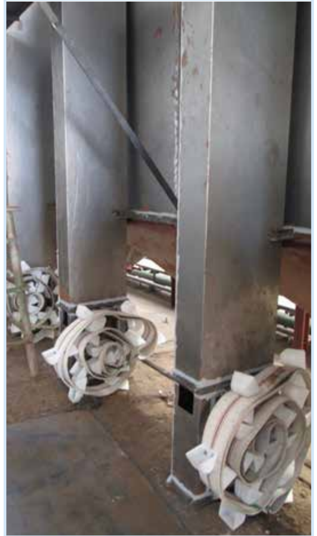
A battery of friction driven bucket elevators used in elevating tea leaves
