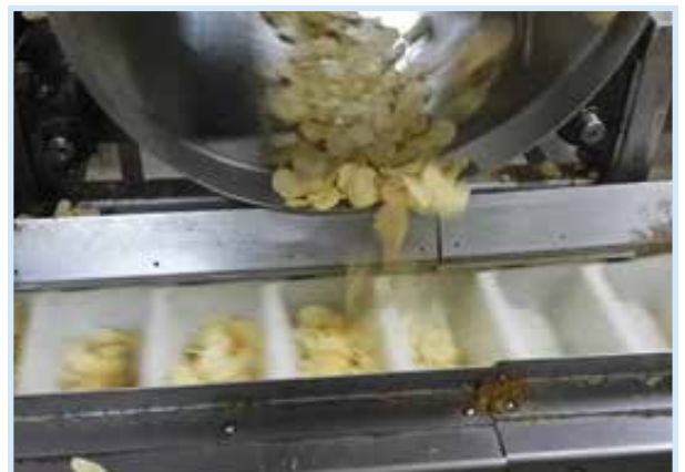
Chain driven continuous buckets shown at infeed in the snacks industry
