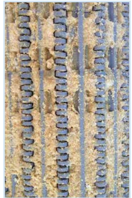
Bottom side of a modular belt
