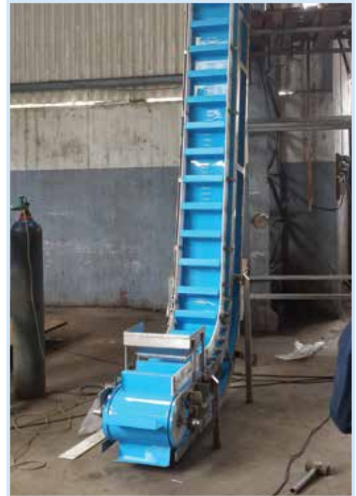
Fixed conveyor side wall
